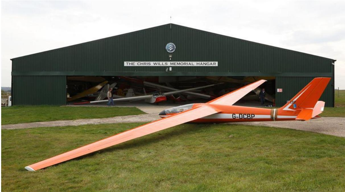
(21<sup>st</sup> April taken by Paul Haliday. The strange markings just in front of the fin are in fact lead weights to keep the glider balanced when it was towed across from outside the VGC hut after rigging!)
